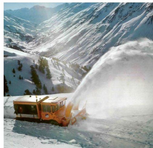
Schmidt snow blower VF3 mounted on an Unimog U406 at work on Timmelsjoch including breathtaking view.
