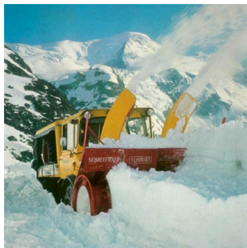
Schmidt snow blower VF3 mounted on an Unimog U406 at work on Timmelsjoch including breathtaking view.
