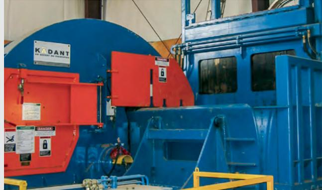
**Disc and ring stranders** cut logs into strands for engineered wood applications including OSB.
